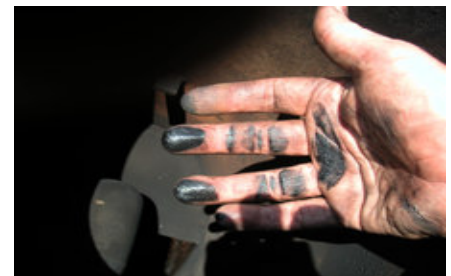
2. Inside the scrubber after the first incident the interior was dry with only carbon residue; however, there was oil in the inlet pipe from the primary compressors.
