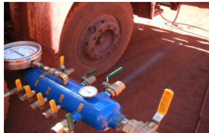
6. Shot of the oil carryover visible as a faint blue mist during another testing. The level of carryover requires LESS than 1 litre of oil per week and can sustain fire.
