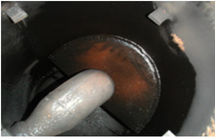
4. Film of oil on the interior of the scrubber after the incident. During testing, the fact that this was still in place is testament to the value of well-placed observers and good emergency shutdowns.
